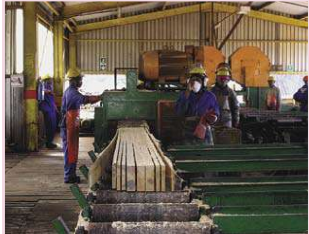
This small pine sawmill in Southern Africa has a much higher recovery of timber compared to a mobile mill.
