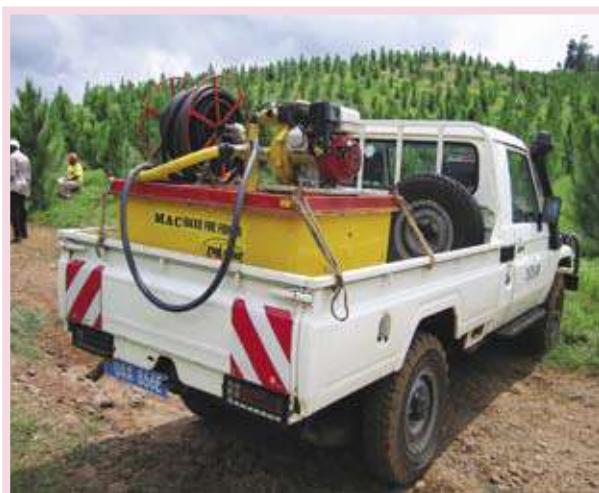
A bakkie-sakkie - 500 lt portable tank and pump (NFA, 2005)
