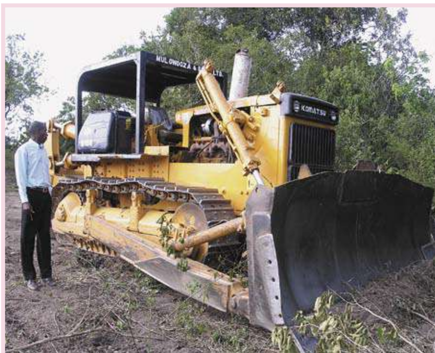
Mechanical land clearance can be very cost-effective if well planned
