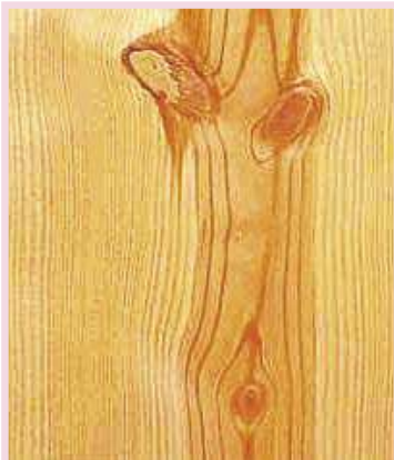
Knots are generally considered as defects in timber.
