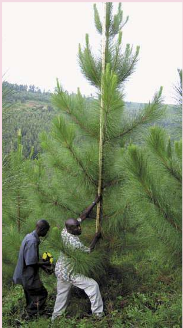
Trees up to 6m are best measured with a height rod (SPGS Training Course, Kyenjojo, 2006)
