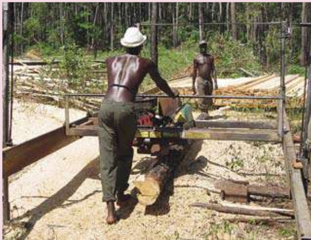
A Lucas mobile saw-mill operating in Katugo CFR (2004). These machines are very inefficient for processing plantation logs.
