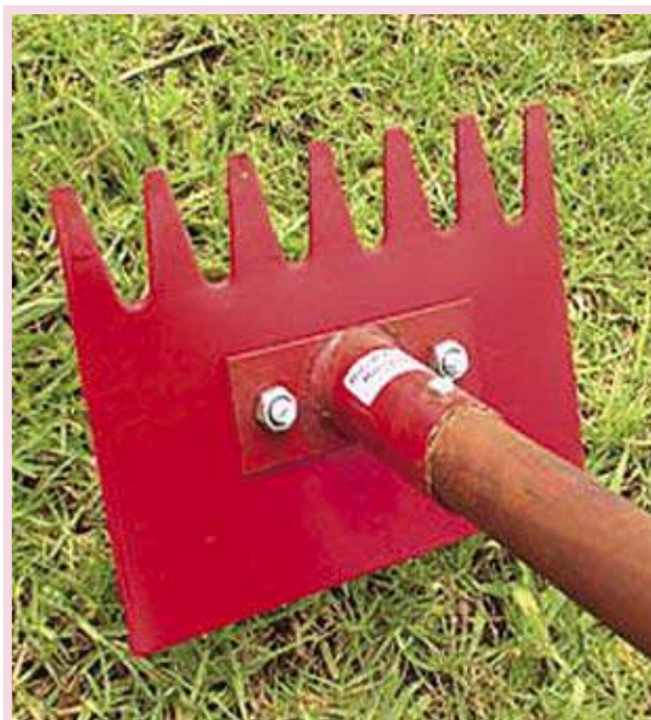
A rake-hoe is useful for clearing firebreaks ahead of a fire.
