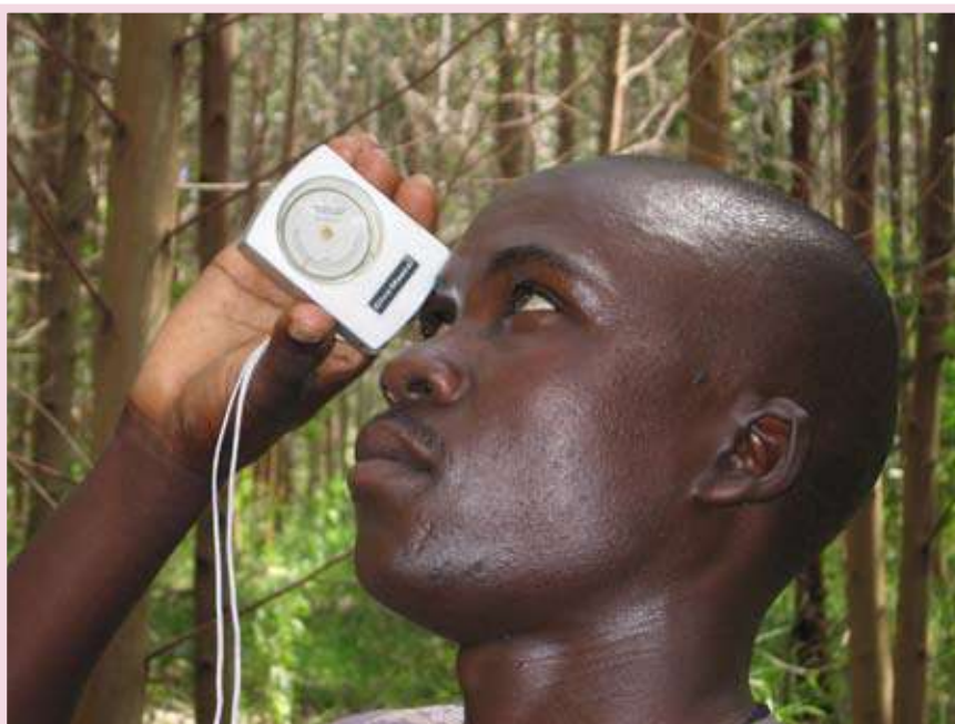
Using a Suunto clinometer to measure tree heights: keeping both eyes open is a challenge !
