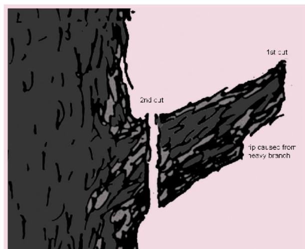
The 2-cut procedure for cutting heavy branches.
